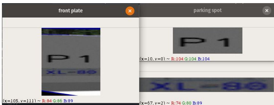
Figure 8: Perspective transformed images showing the extracted license plates and parking spot number from the above saved images
